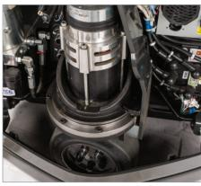
The Brake Is Automatically Engaged When The Truck Isn't
